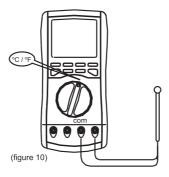
The °C measurement range is  $-40^{\circ}C \sim 1000^{\circ}C$  while °F measurement range is  $-40^{\circ}F \sim 1832^{\circ}F$ . To measure temperature, connect the Meter as follows:
